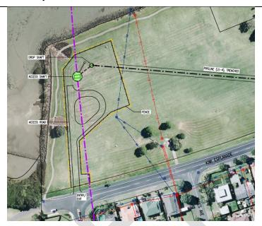
· Access shaft location minimises distances for maintenance workers in section under harbour.
